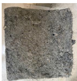
Figure 6. Fiber distribution of the cross-section of the specimen
