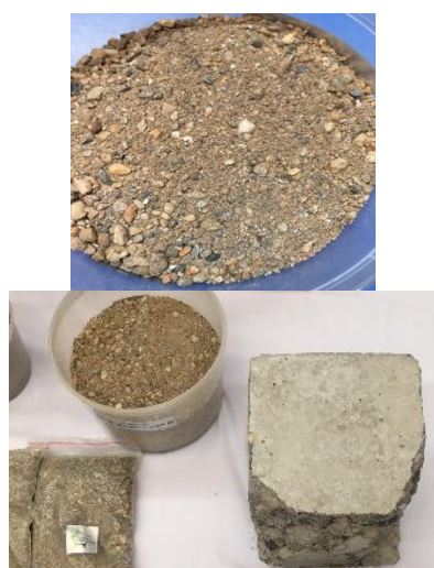
Figure 2. Artificial sand and concrete specimens after compressive strength testing
