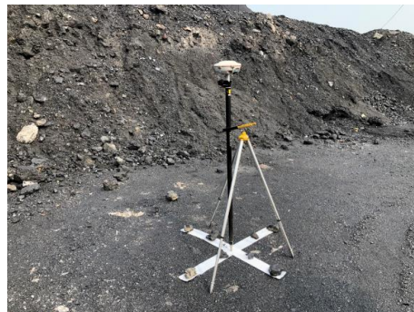
Figure 4. GCPs determination by GNSS/T300
