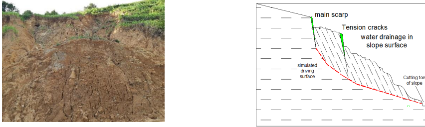
Figure 13. An example of complex type of soil sliding and flow (MCC19 and model)
